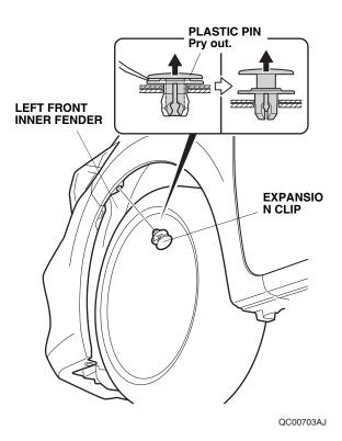
3. Pry out the plastic pin of expansion clip, and remove the expansion clip that fastens the left front inner fender. Retain the expansion clip, then clean the area around the hole.
