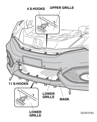
11. Attach six S-hooks to the bottom of the front bumper.
