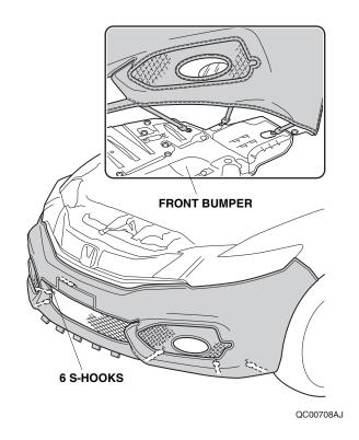
12. Route the elastic cord through five loops on the bottom of the mask. Attach one S-hook to the bottom edge of the bumper on one side. Stretch out the cord after routing it through each loop, then attach the other S-hook to the bottom edge of the front bumper on the other side.
